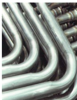
Figure 1: 409 SS exhaust components (photo courtesy of Calsonic, North America Inc)
