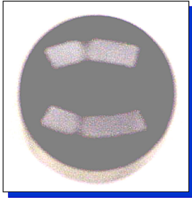
Weld seam before normalizing – Change in metallurgical structure is quite visible
