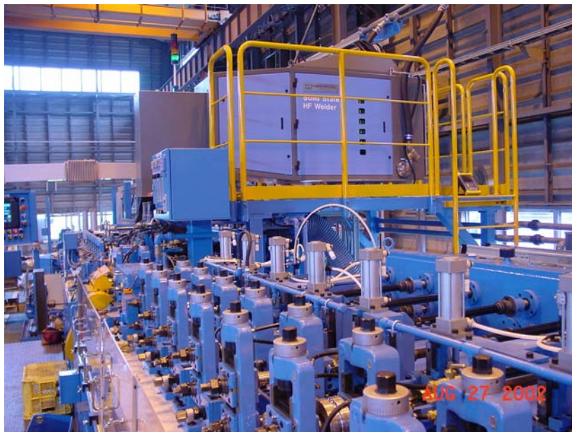
Figure 3 - Typical High D/t Ratio Tube Mill
