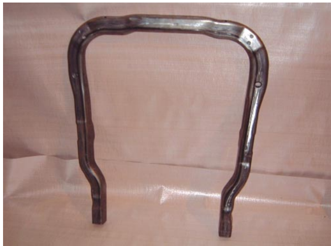
🔗 Crossmember from tube 73x1,30 Source: Aceralia Transformados, GESTAMP HB Hidroacero
