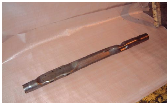
🔗 Crossmember from tube 73x1,30 Source: Aceralia Transformados, GESTAMP HB Hidroacero
